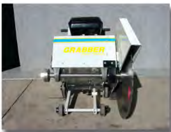
13.5 HP Push Saw with 24" Blade
